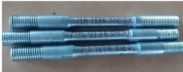
Figure 3: AA 7178/ Wt of 3% SiC Specimens for Hot Tensile Test.
