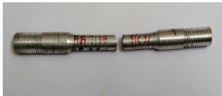
Figure 6: AA 7178/SiC Tested Specimen.
