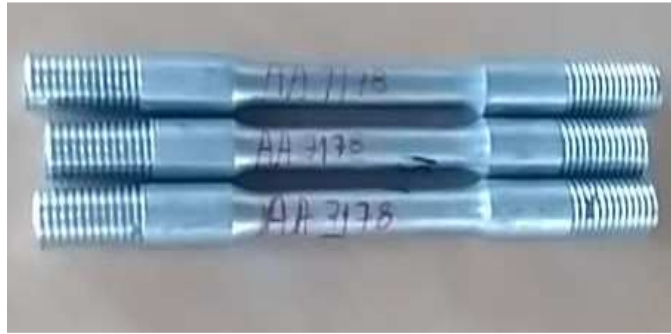
Figure 2: AA 7178 Specimens for Hot Tensile Test.
