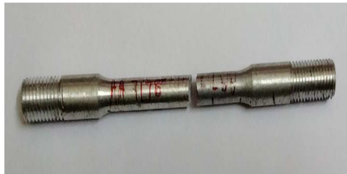
Figure 5: AA 7178 Tested Specimen.
